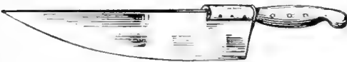
A piece of wood fitted on to the back of a knife-blade saves pressure on the hand
